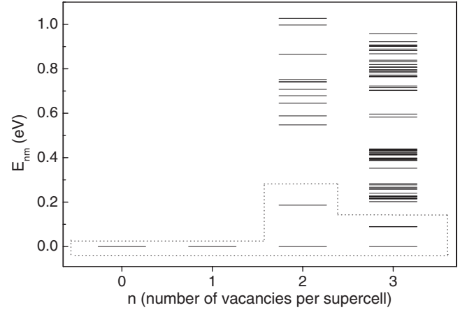
FIG. 2. Configurational energies (relative to the lowest energy at each composition) in the 2 \times 2 \times 2 supercell \text{Mg}_{16}\text{H}_{32-n} . The dotted lines enclose the configurations for which a separate statistical treatment, including vibrational contributions, was performed.
